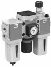
Filter + Regulator + Lubricator Combinations + Poly bowl 5 micron element, 8 bar (116 psig) Regulator + Gauge and Wall Mounting Brackets Inlet pressure 10 bar (145 psig), Secondary pressure 6.3 bar (91.3 psig), 1 bar (14.5 psig) pressure drop.
